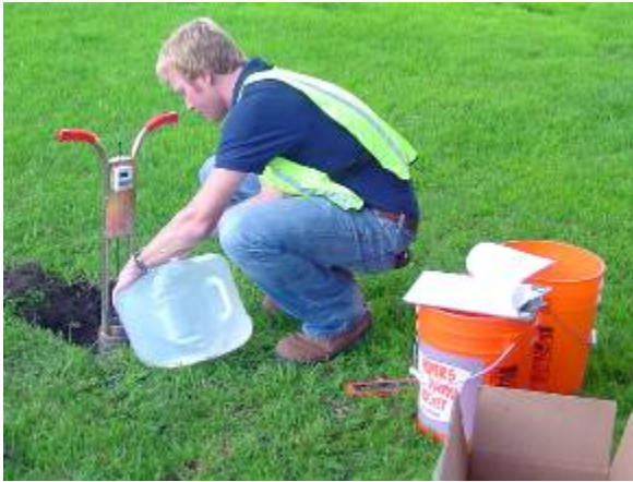
Figure D-3. Infiltrometer Test Setup
