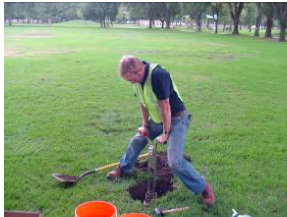
Figure E-2. Sealing the Rings
