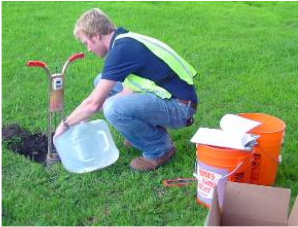
Figure E-3. Infiltrometer Test Setup
